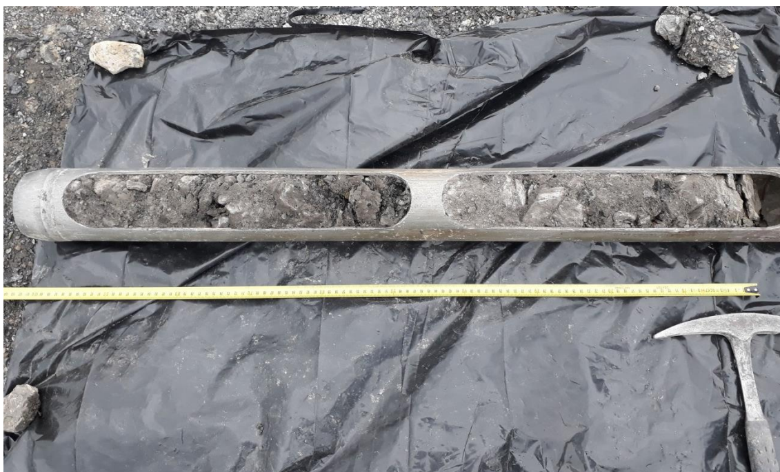
Figure 5 Mine waste profile from Janina Mine spoil heap
