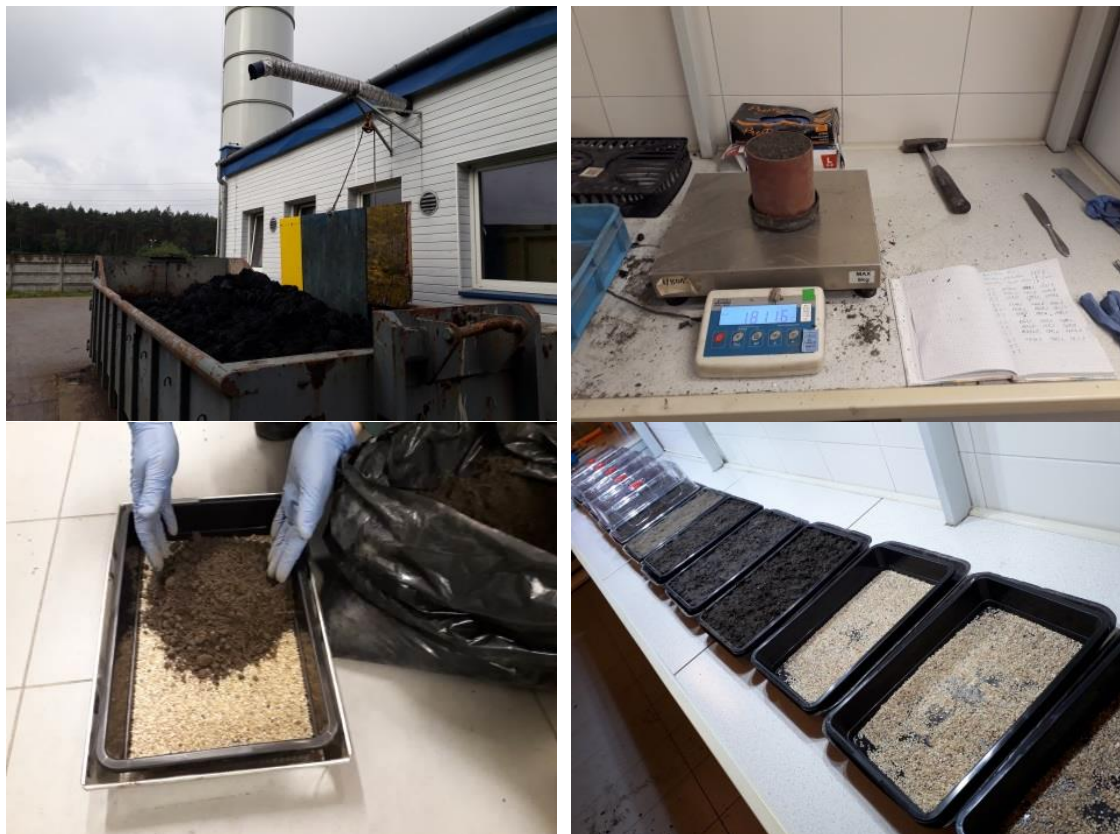
Figure 8 Preparation of soil substitutes in laboratory condition
