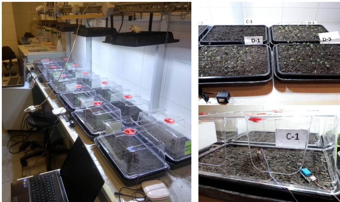
Figure 9 Soil substitutes with Sinapis alba seeds during laboratory phytotoxicity tests
