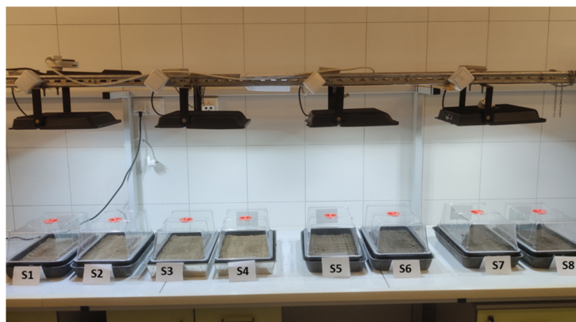
Figure 3. Soil substitutes with Sinapis alba seeds during laboratory phytotoxicity tests.
