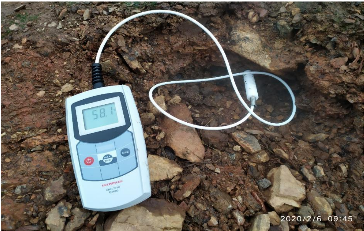
Figure 70. Temperature measurement at the sampling point
