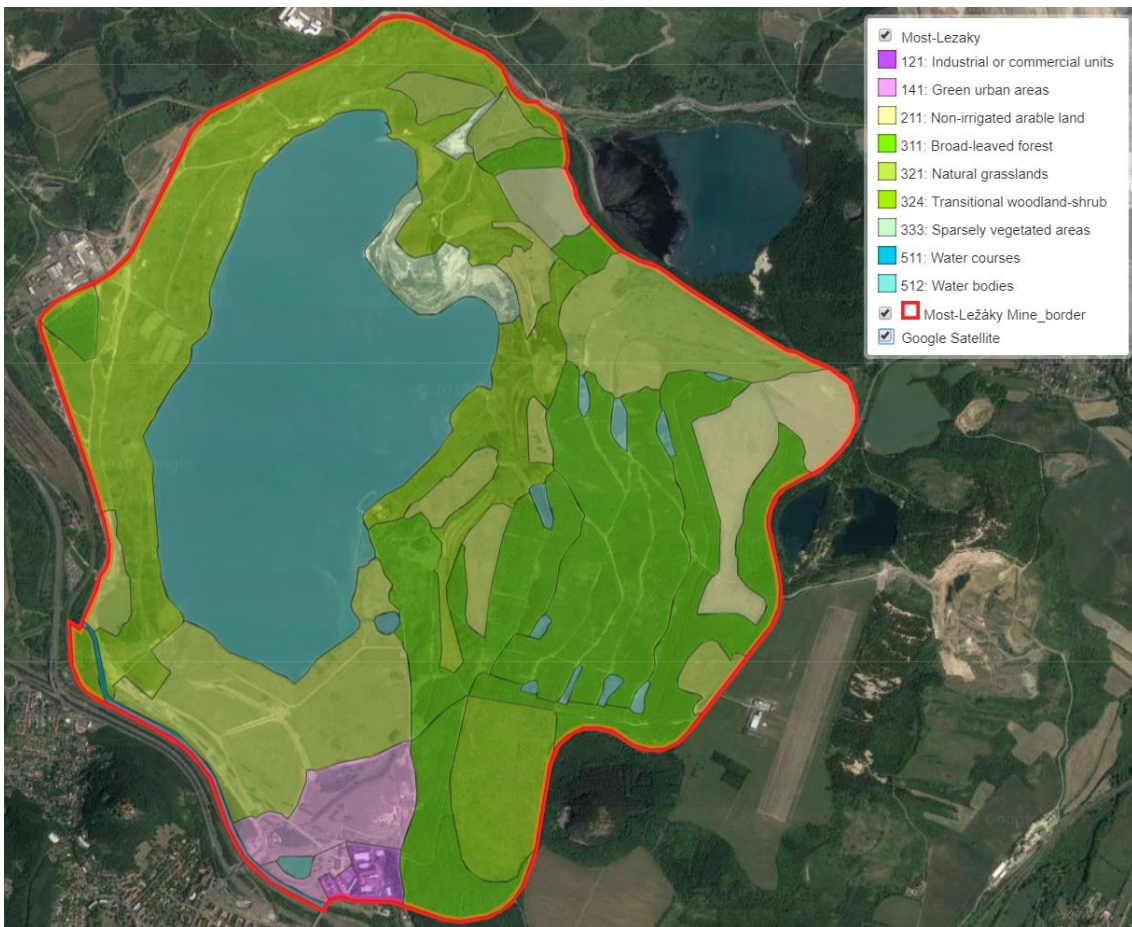
Figure 9-2. GIS presentation of CLC classes in Most-Ležáky over the orthoimage of the area
