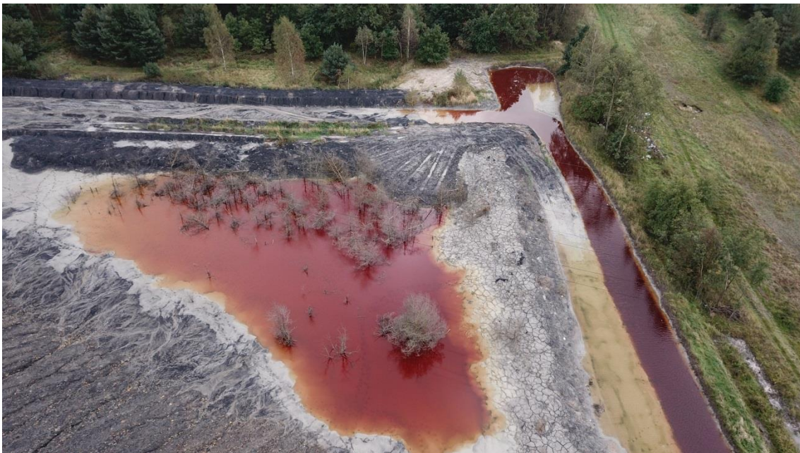
Figure 3-4. Janina Mine Waste Heap – acid rock drainage generation
