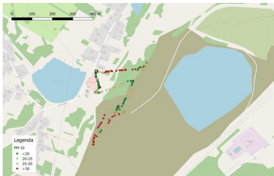
Figure 3-3. Measurement of air pollution spreading from Janina Mine Waste Heap
